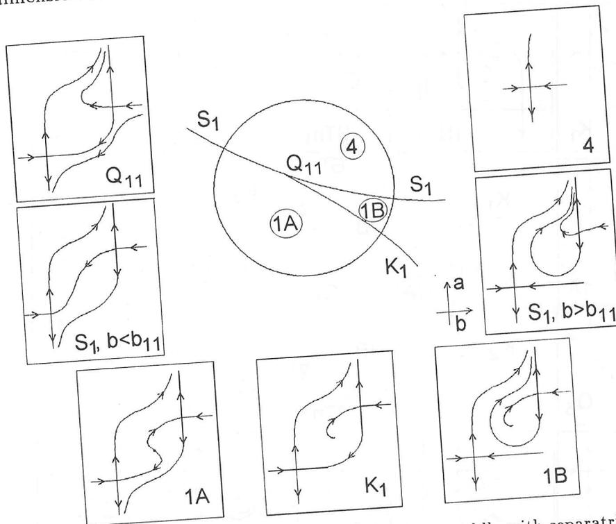
Fig. 8. Bifurcation diagram for the saddle-node–saddle with separatrix connection bifurcation. Here the saddle-node equilibria are partially repulsive
